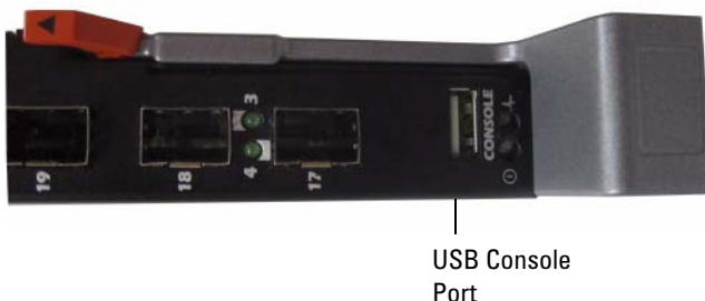
Figure 1-4. PowerConnect M8024-k USB Console Port
